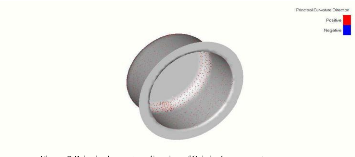
Figure 7. Principal curvature direction of Original component
