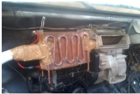
Fig.13 Thermoelectric module fitted to the blower
