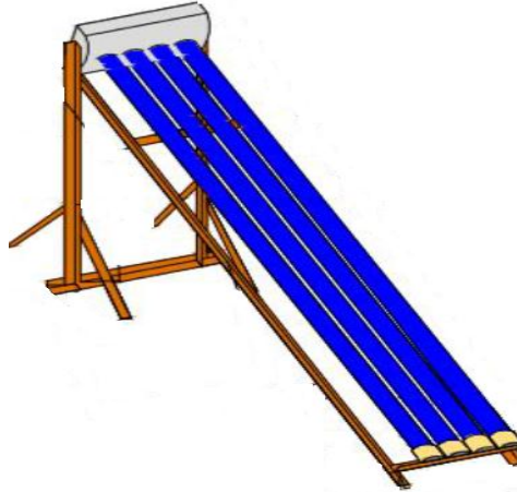
Fig. 3: Solar water heater
