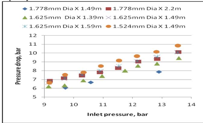
Fig. 2 Variation of Pressure drop with inlet pressure for different capillary
