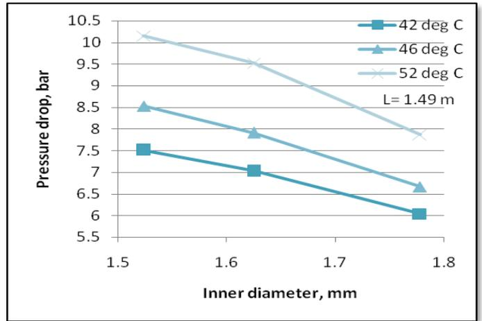
Fig. 4 Variation of pressure drop with inner diameter at constant length
