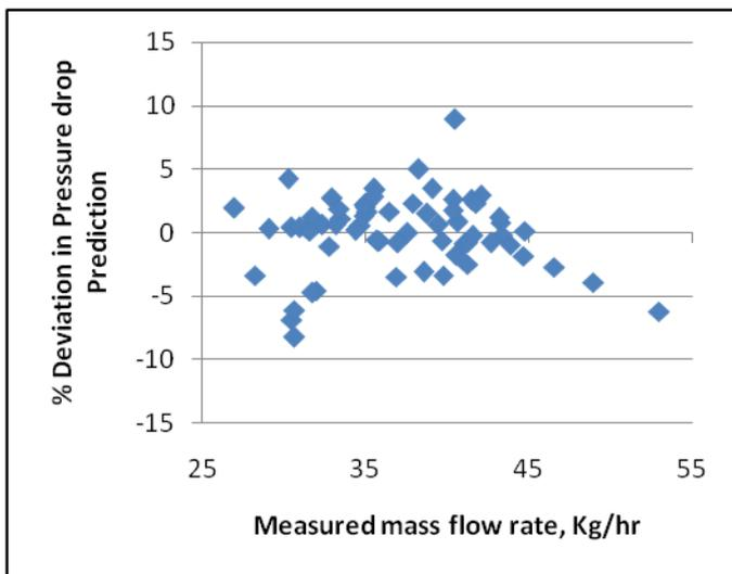
Fig. 7 Deviation in predicted mass flow rate from measured data for different mass flow rate
