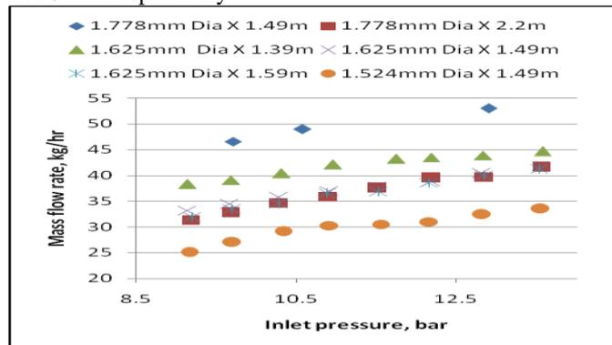
Fig. 3 Variation of Mass flow rate with inlet pressure for different capillary
