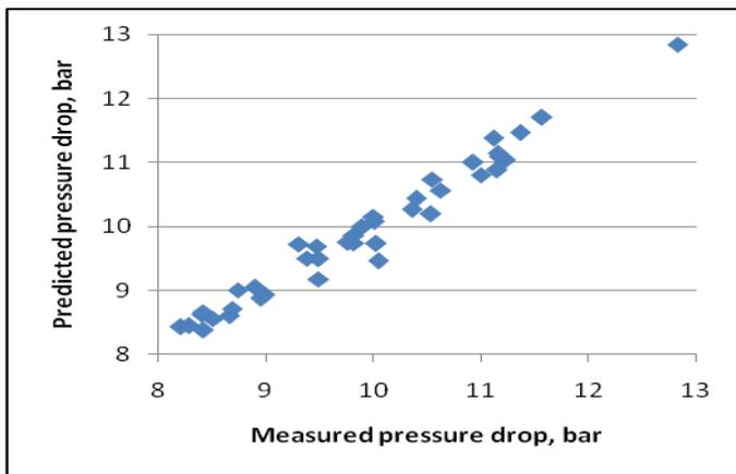
Fig. 6 Comparison of predicted pressure drop with measured pressure drop data with this study
