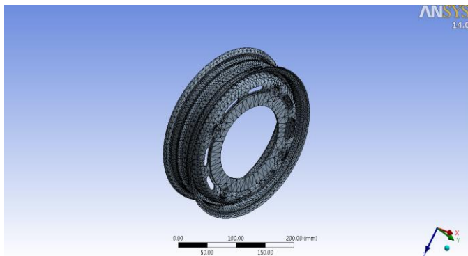
Fig.11 Meshing of wheel rim assembly
