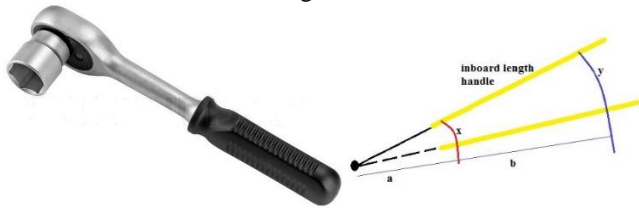
Fig.8 Ratchet and left hand side oar showing backlash Fig 8 shows that 'a' is length of spanner handle and 'b' is extension to spanner handle of inboard length. As arm length increases from 'a' to 'a+b', the arc length increases from 'x' to 'y'. While drive stroke at catch handle will move without any load on it. Therefore this arrangement of belt drive and pulley system is rejected.
