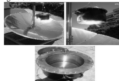
Fig.3.8 (a) Cooker in operation. (b) Focused sun on utensil. (c) Inner pot view with water.
