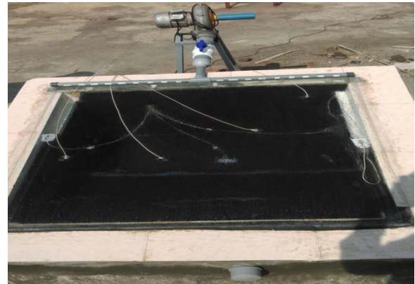
Fig 1. Photograph of Masonic Solar Still
