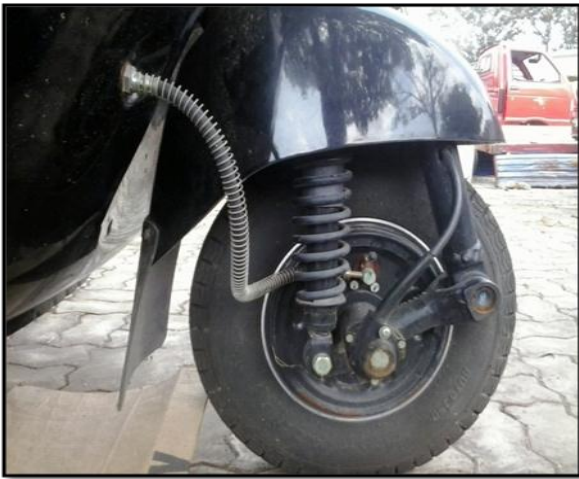
Fig. 3.2: Competitor Trailing Link Suspension
