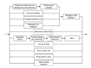
Every function can be accomplished by several alternative principles, e.g. mechanical and thermal principles for weed removal.
